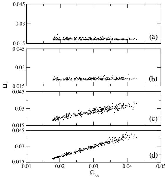
Fig. 3. Bursting frequency for the scale-free lattice versus the zero-coupling frequencies for (a)  $\epsilon = 0.10$ ; (b)  $\epsilon = 0.07$ ; (c)  $\epsilon = 0.03$ ; and (d)  $\epsilon = 0.01$ .
