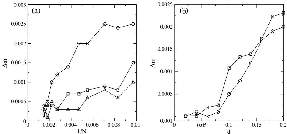
**Fig. 6.** (a) Width of the frequency-locking interval versus inverse lattice size for  $N_p = 1$  driving signal, applied to the most connected site (circles), the second (squares) and the third (triangles) most connected sites, with amplitude  $d = 0.20$ . (b) Tongue width as a function of the driving amplitude for (a)  $N_p = 1$  driving signal applied to the most connected site; (b)  $N_p = 10$  driving signals applied to randomly chosen sites.
