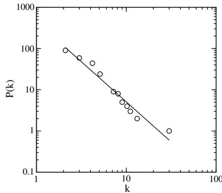
Fig. 1. Probability distribution for the connectivity of the final scale-free lattice with  $N = 230$  sites. The solid line is a least-squares fit with slope  $-2.08$ .
