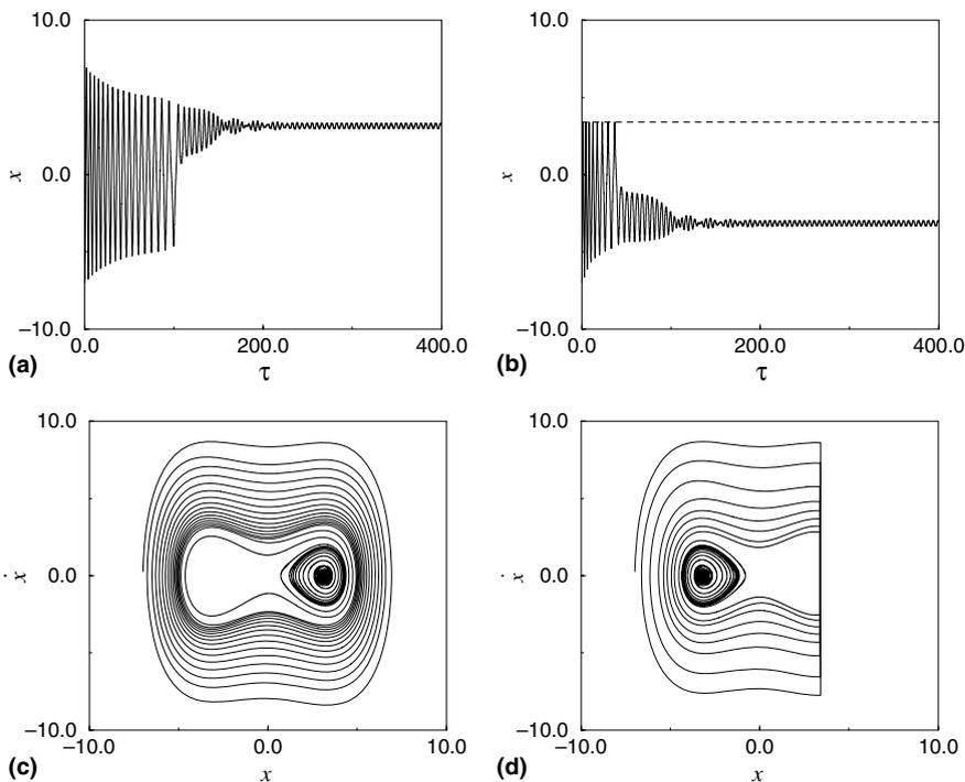
Fig. 7. Displacement versus time of the attractors  $A$  and  $B$  shown in Fig. 3(a); (a) attractor  $A$  without impacts; (b) attractor  $B$  with impacts (at  $x_c = 3.4$ , dashed line) during the transient regime, (c) and (d) shows the corresponding phase space trajectories of (a) and (b), respectively.
