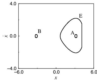
Fig. 8. Velocity versus displacement of the cart for three periodic attractors at  $E_1 = 1.7$  and  $x_c = 4.1$ .
