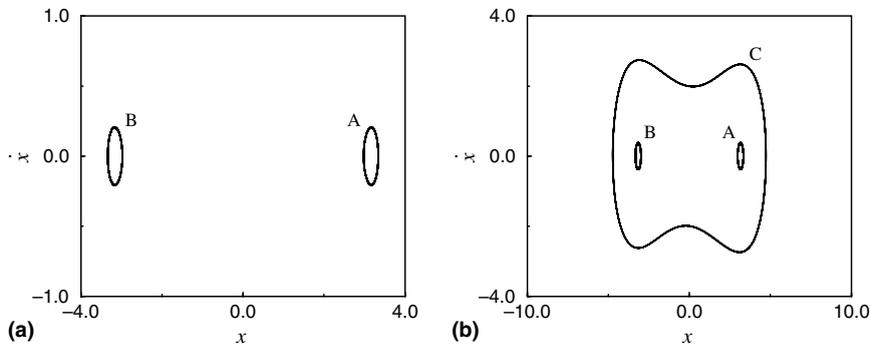
Fig. 3. Velocity versus displacement of the cart. (a) Two periodic attractors for  $E_1 = 1.70$ ; (b) Three periodic attractors for  $E_1 = 3.25$ .
