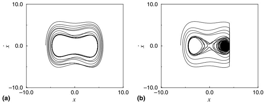
Fig. 11. Phase space trajectories corresponding to the attractor  $E$  of Fig. 5(b). (a) Without constraints, (b) with a constraint at  $x_c = 4.1$ .
