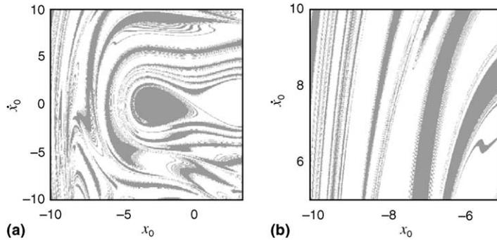
Fig. 6. (a) Basins of attraction of the two periodic attractors  $A$  (white) and  $B$  (gray) shown in Fig. 5(a) for  $x_c = 3.4$  and (b) their magnification.
