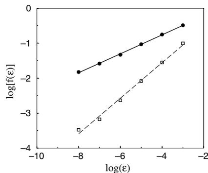
Fig. 12. Uncertain fraction versus  $\epsilon$  for the basin boundary region depicted in Figs. 4(b) (solid line) and 6(b) (dashed line). The lines are least squares fits, with slopes  $0.27 \pm 0.01$  (solid line) and  $0.51 \pm 0.02$  (dashed line).
