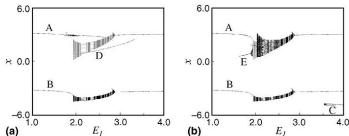
Fig. 5. Bifurcation diagrams showing the attractors of the cart displacement as a function of the control parameter  $E_1$ . (a) For  $x_c = 3.4$  and (b)  $x_c = 4.1$ . In gray is shown the attractors without impacts (the same are labelled  $A$  in Fig. 2).
