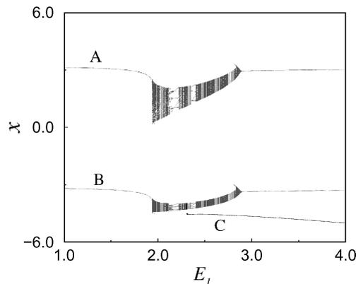
Fig. 2. Bifurcation diagram showing three attractors of the cart displacement without impacts as a function of the control parameter  $E_1$ .
