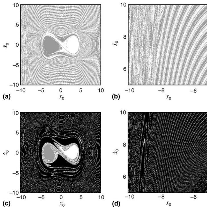
Fig. 4. Basins of attraction, (a) for the two periodic attractors  $A$  (white) and  $B$  (gray) shown in Fig. 3(a), (b) magnification of previous figure, (c) for the three periodic attractors  $A$  (white),  $B$  (gray),  $C$  (black) shown in Fig. 3(b), (d) magnification of previous figure.
