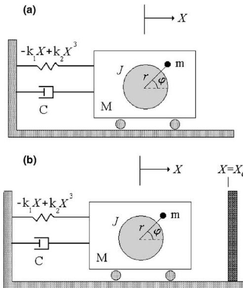
Fig. 1. (a) Schematic model of a cart driven by a motor with unbalanced mass; (b) model with a limited constraint.
