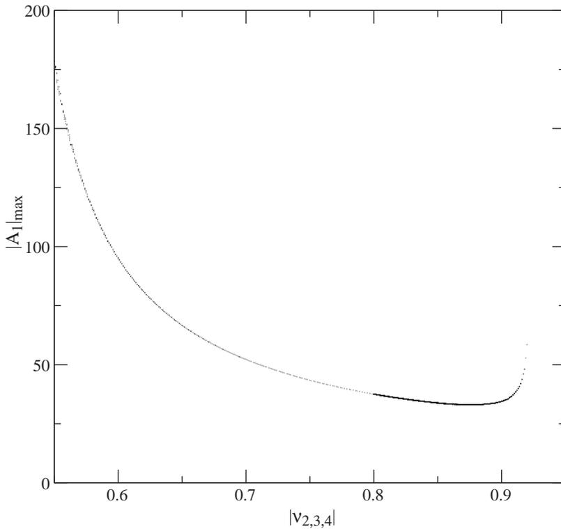
Fig. 13. Bifurcation diagram of the system as a function of  $v_{2,3,4}$  for  $\Delta = 0$ .
