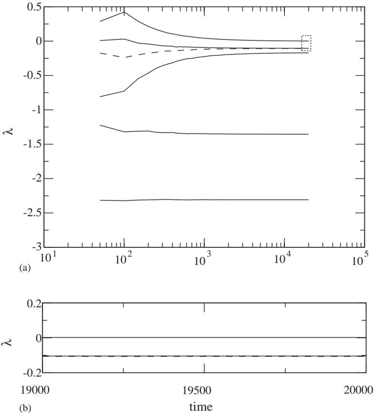
Fig. 6. (a) Time evolution of the Lyapunov exponents for the resonant four-wave parametric interaction  $\Delta = 0.01$  and  $v_{2,3,4} = -0.8$ . (b) Magnification of (a).
