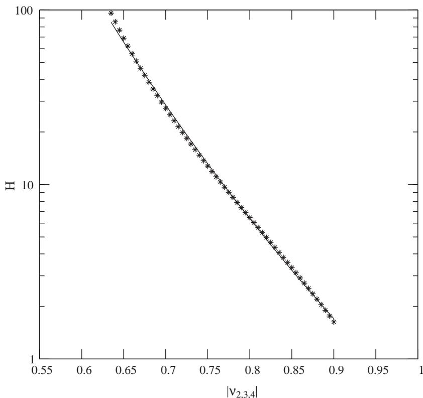
Fig. 11. Asymptotic energy function ( $H(t)$ ) as a function of the dissipative parameters  $v_{2,3,4}$  for  $\Delta = 0.0$ .
