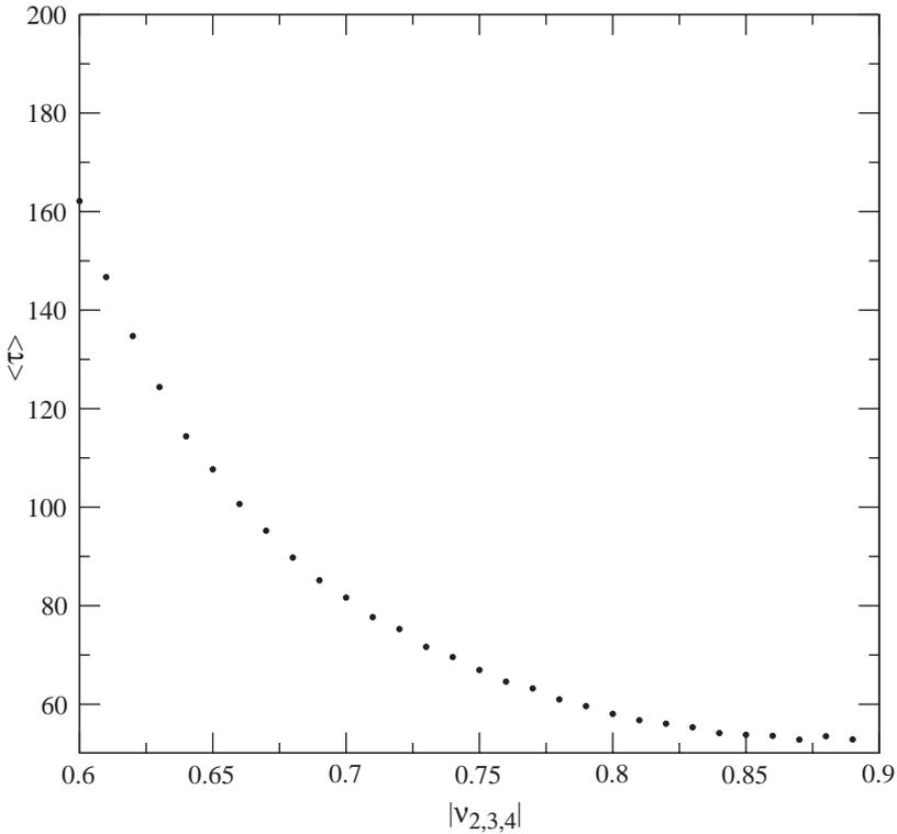
Fig. 12. Average transient time over 500 initial conditions for the system settles down in the invariant manifold as a function of the dissipation parameters  $v_{2,3,4}$  for  $\Delta = 0$ .
