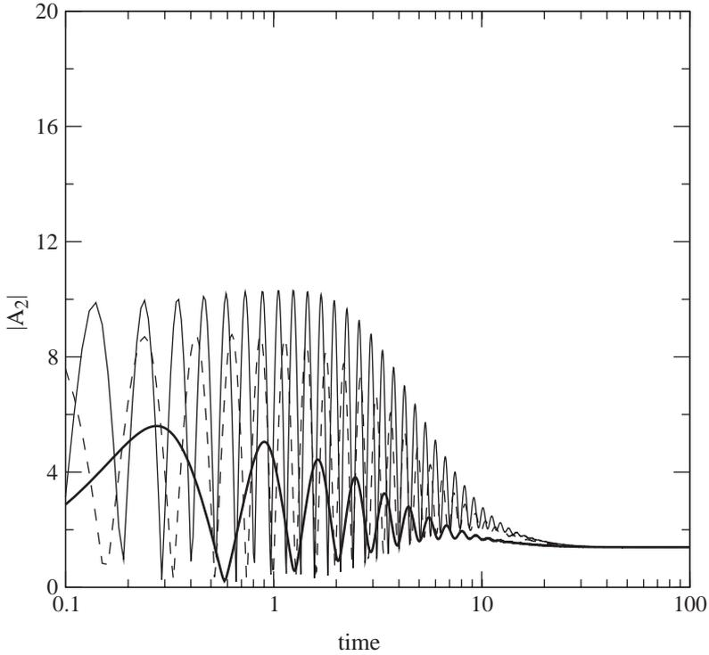
Fig. 2. Time evolution of wave 2 amplitude for the resonant four-wave parametric interaction for  $\Delta = 0$  and  $\nu_{2,3,4} = -0.8$ .
