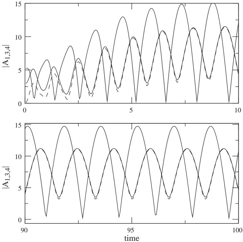
Fig. 3. Time evolution of waves 1, 3 and 4 for the resonant four-wave parametric interaction for  $\Delta = 0$  and  $\nu_{2,3,4} = -0.8$ .
