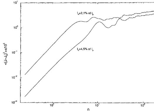
**FIGURE 2.** Time evolution of the mean square action deviation for two different EML currents, and a bunch of initial conditions depicted in Fig. 3a, for the same parameters of Figs. 1a and 1b.  $n$  is the number of toroidal turns
