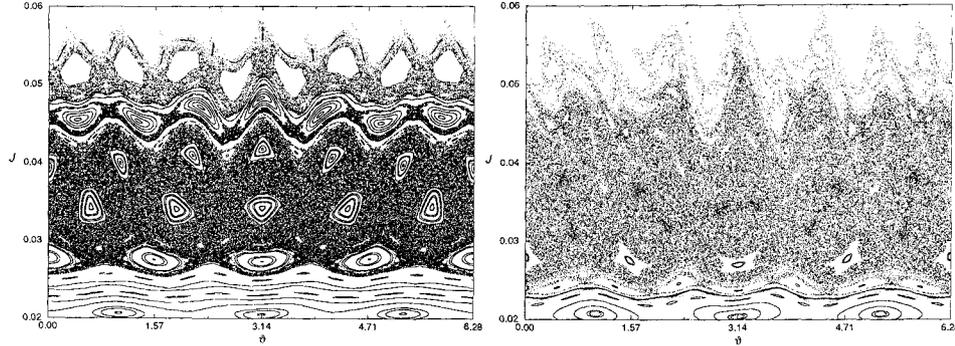
**FIGURE 1.** Stroboscopic field line map for  $N_a = 4$  limiters with  $I_h = 0.021I_p$  (a), and  $I_h = 0.045I_p$  (b), with  $(m_0, n_0) = (4, 1)$ , and  $\lambda = 0.4827$ .
