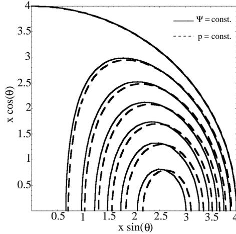
**Figure 3.** Magnetic flux and pressure surfaces for  $\epsilon = 0.2$ ,  $\lambda R = 4$  and  $g_0 = 0$ .
