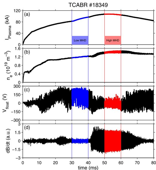
**Fig. 1.** Time evolution of plasma discharge in TCABR tokamak. (a) Plasma current, (b) central chord plasma mean density, (c) floating electrostatic potential for a typical discharge inside the limiter ( $r = 17$  cm), (d) ion saturated current from the vertical lines indicate the analyzed time interval.
