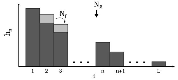
**Fig. 7.** The one-dimensional sandpile model with  $L$  cells versus height  $h_n$ , where  $n$  is each lattice site,  $N_f$  is the number of sand grains that slide off the sandpile slope and  $N_g$  is the number of sand grains randomly deposited at each time.
