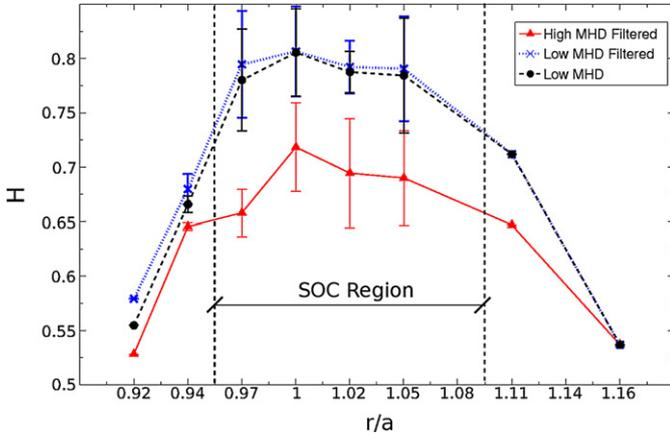
**Fig. 6.** (Color online.) Radial dependence of the Hurst parameter in time range with low MHD activity (circles), high MHD activity filtered (triangles) and low MHD activity filtered (asterisks) with the same spectral range used in high MHD activity. The vertical black dashed lines marks the position of the existence of SOC behavior radial dependence.
