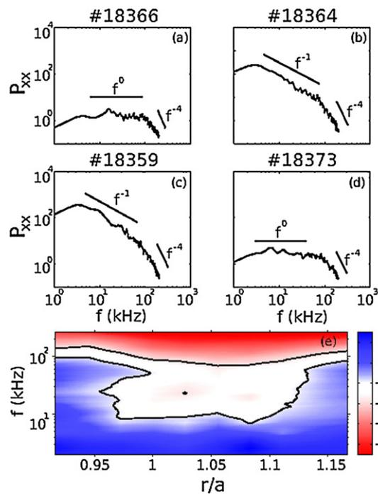
**Fig. 2.** Power spectrum  $P_{xx}$  of the floating potential fluctuation at four different radial positions: (a)  $r/a = 0.91$  (inside the plasma column); (b)  $r/a = 1.00$  (limiter); (c)  $r/a = 1.05$  and (d)  $r/a = 1.16$  (outside the plasma column), respectively. (e) Local decay exponent in function of the frequency and the radial position obtained from 28 shots. (For interpretation of the references to color in this figure, the reader is referred to the web version of this Letter.)
