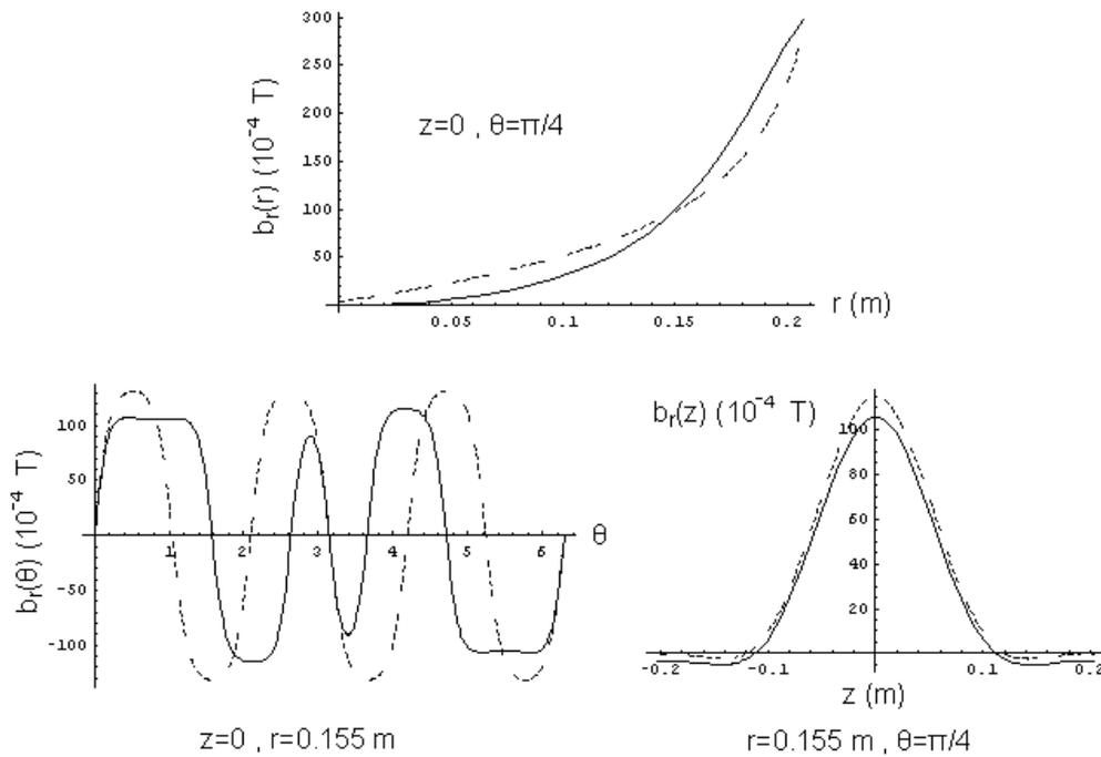
**Figure 6.** Radial component of the ergodic limiter field as a function of  $r$ ,  $\theta$  and  $z$  coordinates separately, the other ones being held fixed, as indicated. The limiter current was considered  $I_L = 2500$  A. The full (dashed) line is for limiter straight segments with non-uniform (uniform) poloidal distribution.
