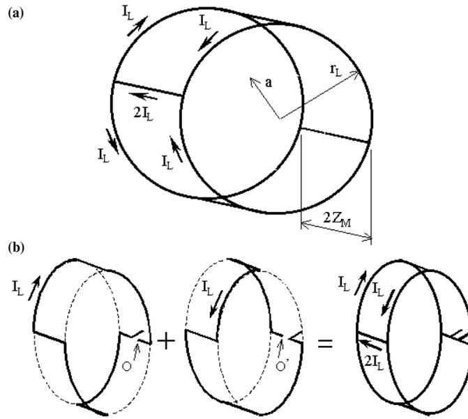
**Figure 2.** (a) Schematic of the  $m = 2$  ergodic magnetic limiter; (b) two conductors are conveniently superimposed to obtain the limiter.
