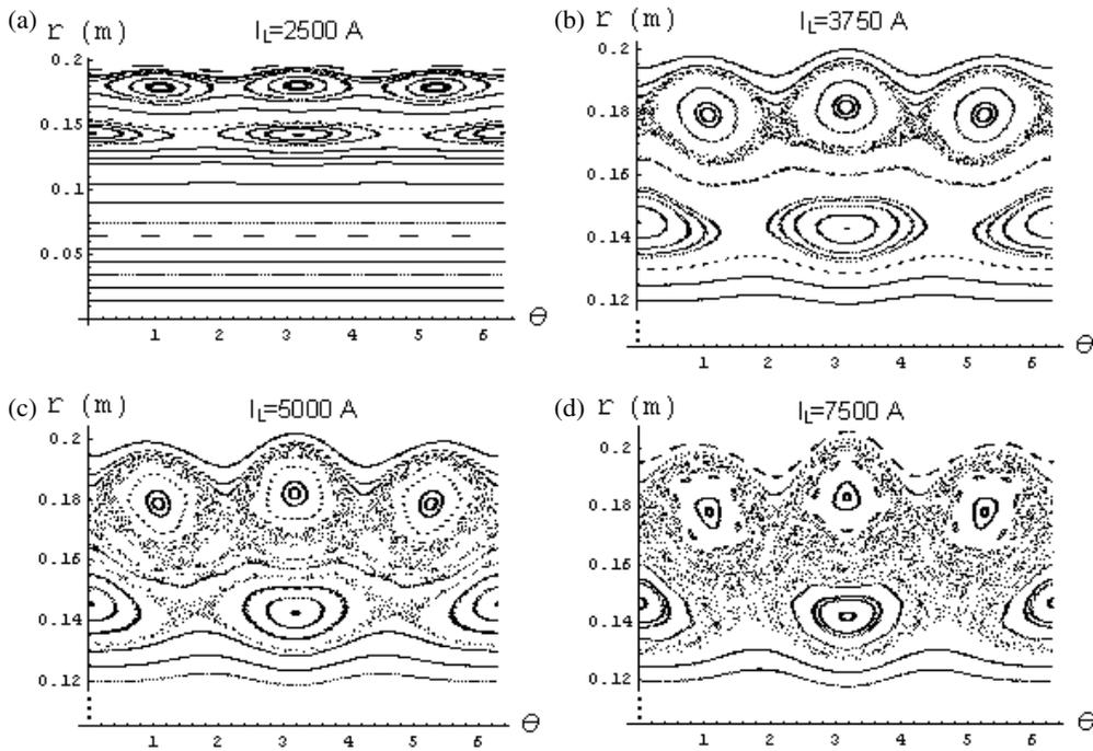
**Figure 11.** Poincaré maps of magnetic field lines in the case of two limiter rings with  $p = 3$  and 2, diametrically opposed, and current (a)  $I_L = 2500$  A, (b)  $I_L = 3750$  A, (c)  $I_L = 5000$  A and (d)  $I_L = 7500$  A.
