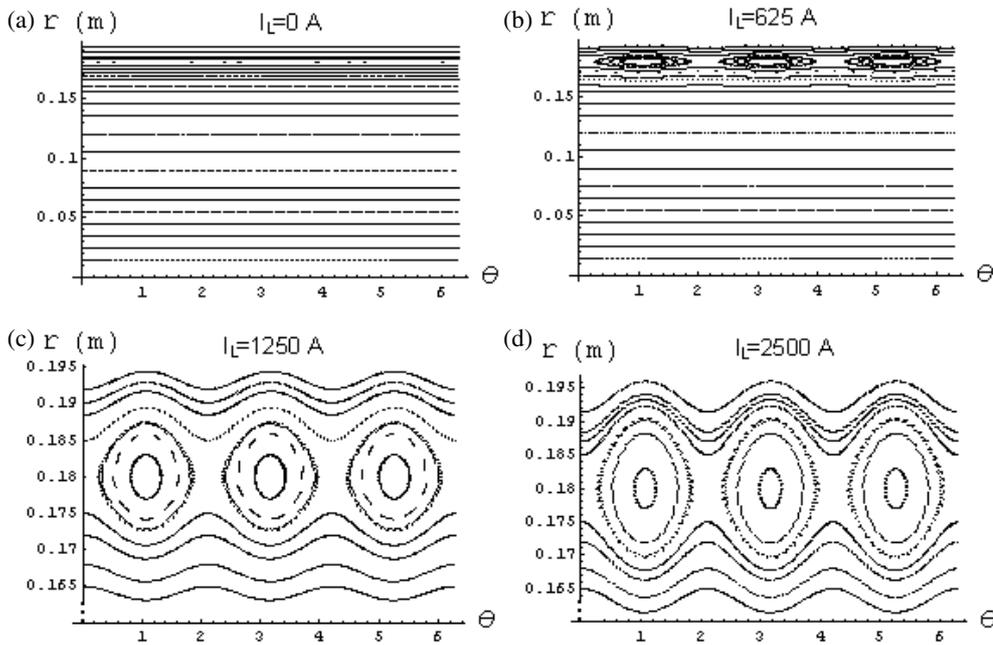
**Figure 10.** Poincaré maps of magnetic field lines in the case of a limiter with  $p = 3$ , a uniform poloidal distribution of straight limiter segments, and currents (a)  $I_L = 0$ , (b)  $I_L = 625$  A, (c)  $I_L = 1250$  A and (d)  $I_L = 2500$  A.
