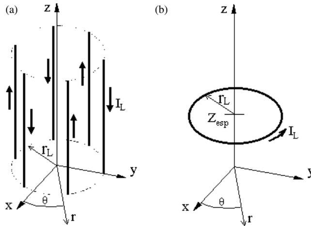
**Figure 4.** (a) Three pairs of infinitely long wires mounted at the limiter position  $r + r_L$ ; (b) a conducting coil of radius  $r_L$  at  $z = Z_{\text{coil}}$ .
