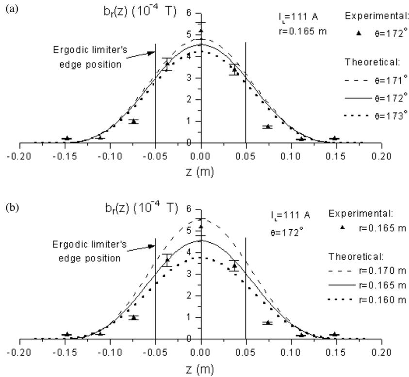
**Figure 9.** Radial component of the ergodic limiter field as a function of  $z$ , for (a) a fixed radial position ( $r = 0.165$  m); and (b) a fixed poloidal position ( $\theta = 172^\circ$ ). The other parameters are held fixed, as indicated. The current through the limiter is  $I_L = 111$  A. The lines are drawn from results obtained with the help of equation (15), and the points plotted are for experimental measurements.
