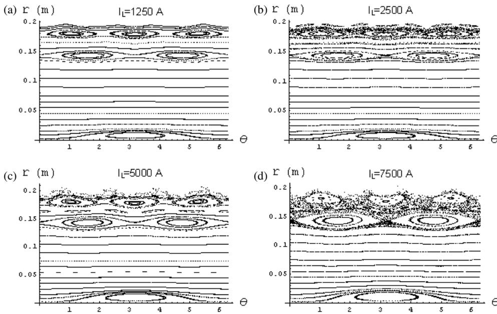
**Figure 12.** Poincaré maps of magnetic field lines in the case of one limiter ring with  $p = 3$ , a non-uniform poloidal distribution of straight limiter segments, and current (a)  $I_L = 1250$  A, (b)  $I_L = 2500$  A, (c)  $I_L = 5000$  A and (d)  $I_L = 7500$  A.
