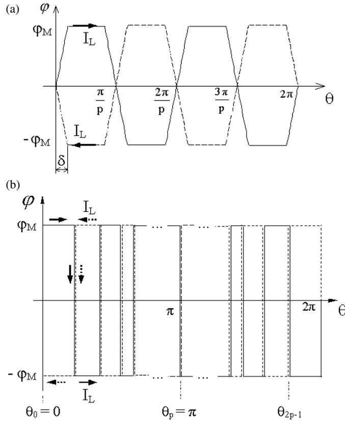
**Figure 3.** (a) Uniform and (b) non-uniform poloidal distribution related to the wire segments of an ergodic limiter.
