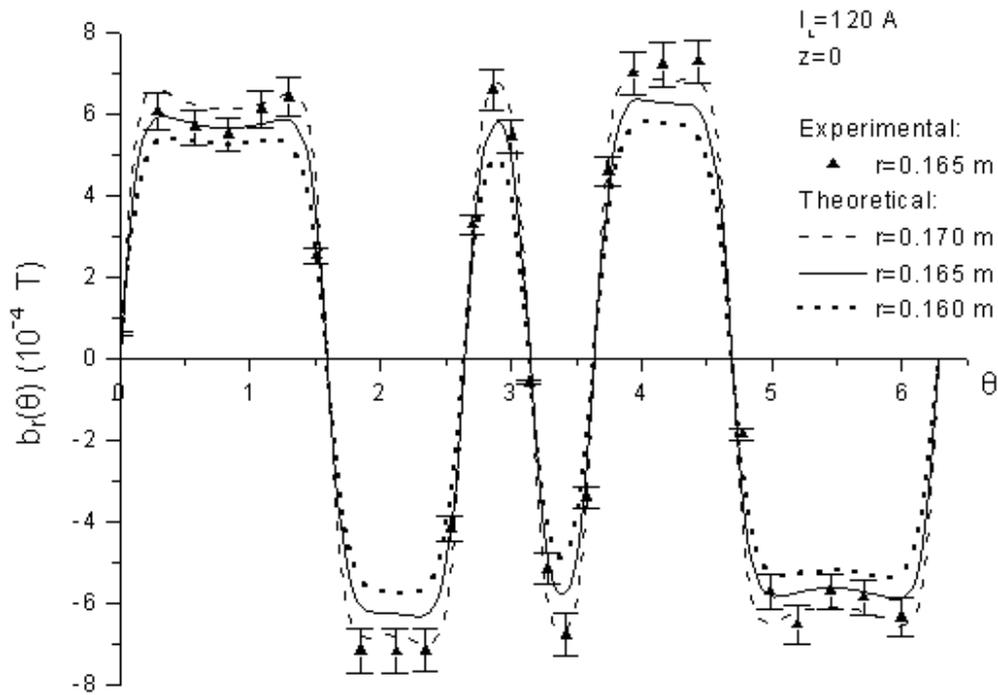
**Figure 8.** Radial component of the ergodic limiter field as a function of the coordinate  $\theta$ , the other ones being held fixed as indicated. The limiter current is  $I_L = 120 \text{ A}$ . The lines were obtained using equation (15), and the points represent the experimental measurements.
