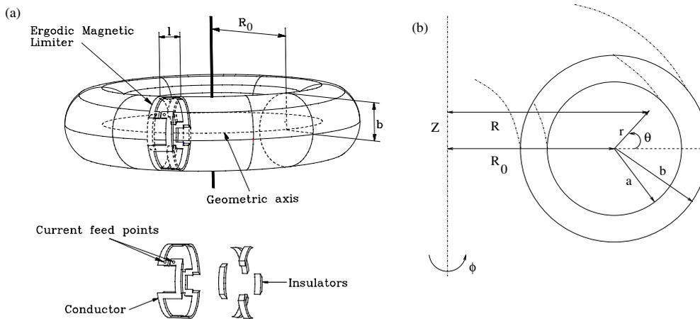
**Figure 1.** (a) Scheme of the ergodic magnetic limiter (reprinted, with permission, from [35]); (b) local coordinates.
