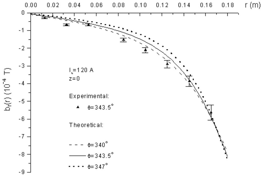
**Figure 7.** The intensity of the radial component of the ergodic limiter field as a function of the coordinate  $r$ , the other ones being held fixed as indicated, for a limiter current  $I_L = 120 \text{ A}$ . The lines correspond to the results yielded by equation (15), whereas the points indicate the experimental measurements.
