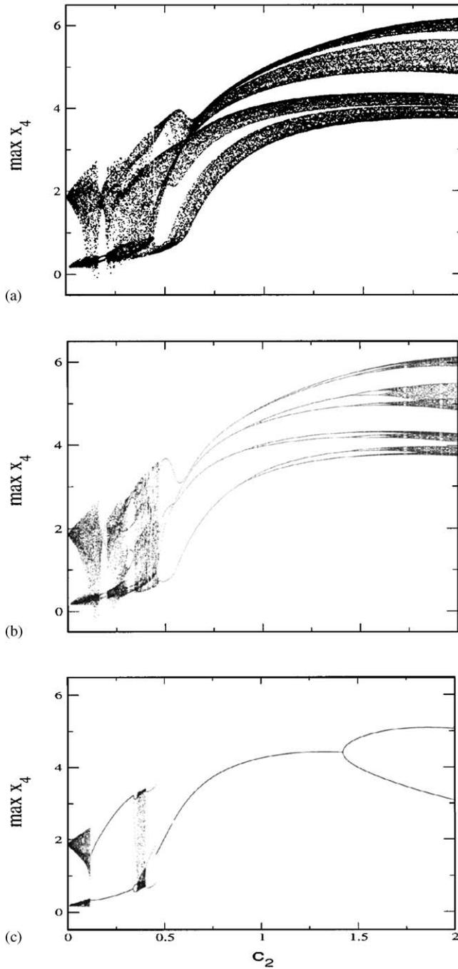
Fig. 11. Bifurcation diagrams for the maximum values of the variable  $x_4$  as a function of the coupling strength  $c_2$  for  $c_1 =$  (a) 0.0; (b) 0.1; and (c) 0.5.
