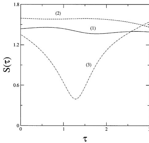
Fig. 6. Similarity function for varying time lag for  $c_2 =$  0.05 (1); 0.12 (2); and 0.48 (3).
