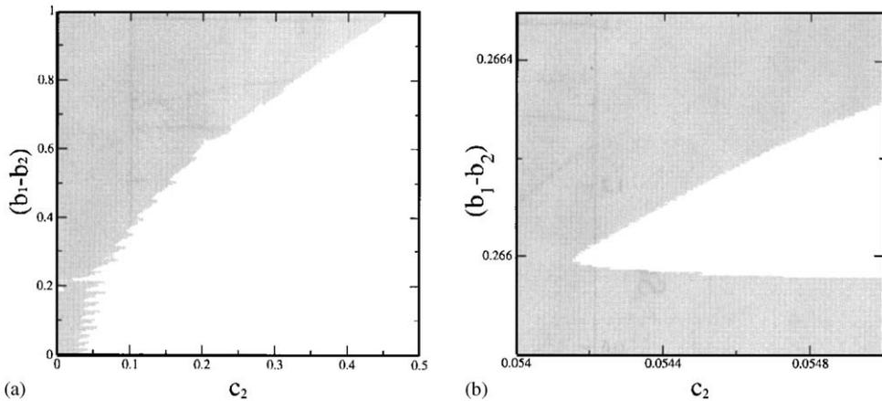
Fig. 7. (a) Synchronization regions in the parameter plane of normal mode frequency mismatch versus coupling strength. White (gray) regions represent parameter values for which the conditional exponent  $\lambda_{cond}$  is negative (positive), (b) Magnification of the tip of one Arnold' tongue.
