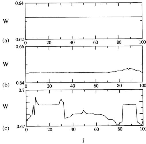
Fig. 2. Frequency profile for a lattice of  $N = 101$  coupled vdP oscillators with  $a = 2.8$ ,  $b = 1.0$ ,  $K = 3.0$ , random initial conditions, periodic boundary conditions, normal mode frequencies randomly distributed over the interval  $[0, 1]$ . (a)  $\alpha = 0.0$ ; (b)  $\alpha = 1.3$ ; and (c)  $\alpha = 1.7$ .
