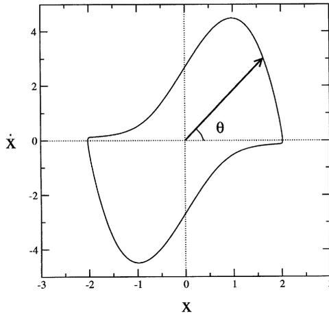
Fig. 1. Phase portrait of an uncoupled vdP oscillator with  $a = 2.8$ ,  $b = 1.0$ , and  $\Omega = 1.0$ , showing how the phase is defined for the system.
