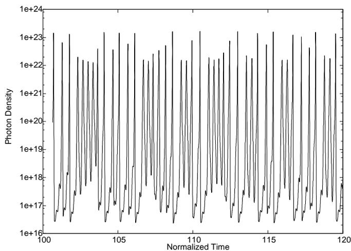
Figure 2: Photon density as a function of time for the chaotic state of the laser diode.
