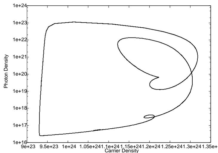
Figure 4: Stabilization of a periodic orbit for the laser diode with the given parameters.
