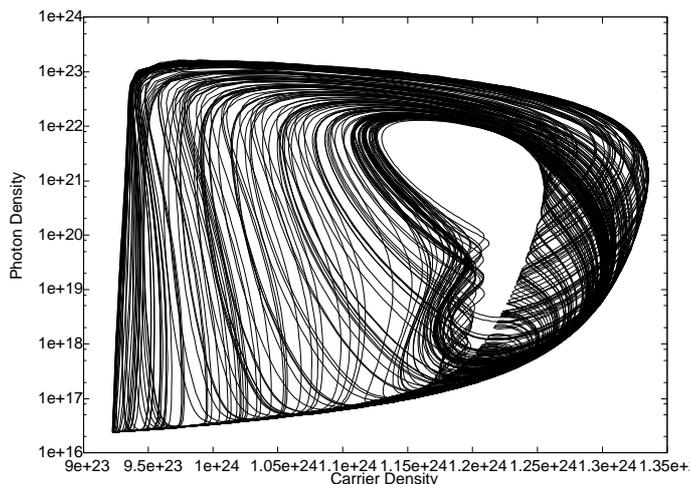
Figure 1: Chaotic attractor for a laser diode under proper bias and modulation current. See text for details.
